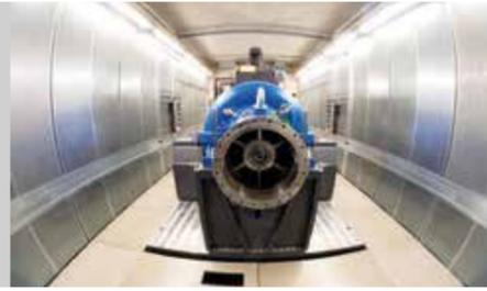
With the test air supply system made by AERZEN, the test benches (here air turbine) can be operated dynamically with almost freely selectable load ramps.
