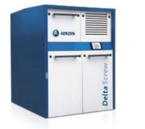
High-efficiency compressor package (single-stage) with belt drive. Optionally with pre-inlet version for high negative pressure up to -850 mbar. Also suitable for suction/ pressure operation. Oil-free as per class O Extremely resilient, durable and lowmaintenance.
