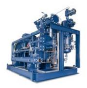
Reliable compressor package with oil-injection. Stepless volume control by hydraulically operated slide valve (slide control). Integrated oil separation, 6 sizes.
