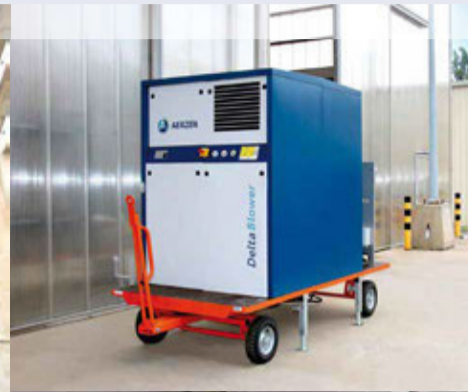
Mobile salt conveyor system in Luxembourg with an AERZEN GM 355 positive displacement blower. A mobile solution was necessary because it was not permitted to change the appearance of the warehouse.
