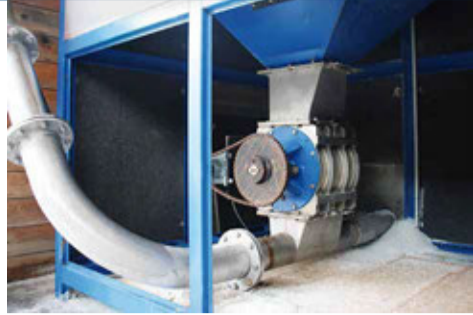
Inside the inlet funnel a rotary valve distributor takes care of the dosage of the salt and the constant throughput. Emde flow-optimised the product inlet.
