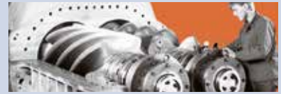
The world's largest screw compressor built for and delivered to the chemical industry
