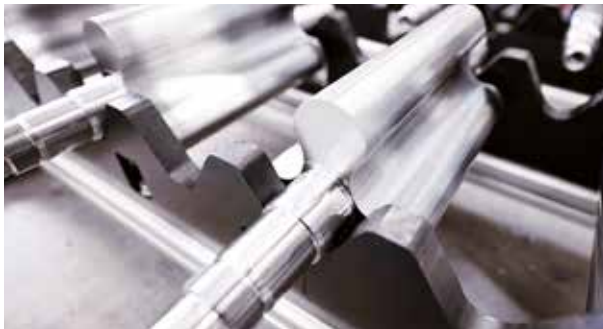
Pure precision: rotary lobes, pre-assembly
