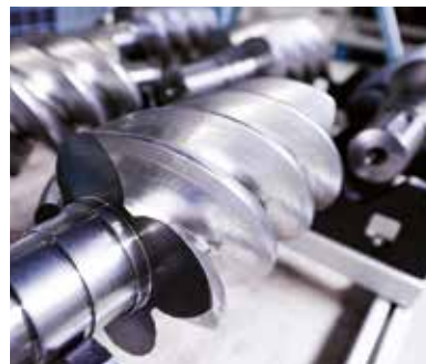
Superior performance at higher pressures: screw compressor rotors
